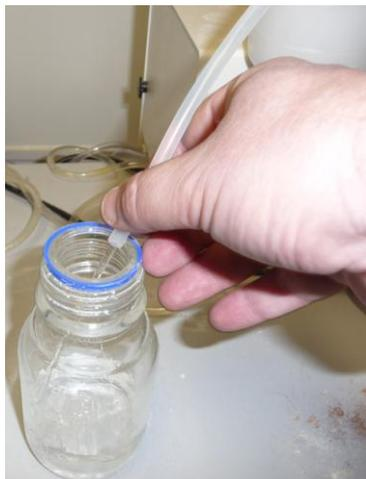
4. Any air bubbles should be purged from the line and a constant stream of fluid should be going into the waste bottle.
